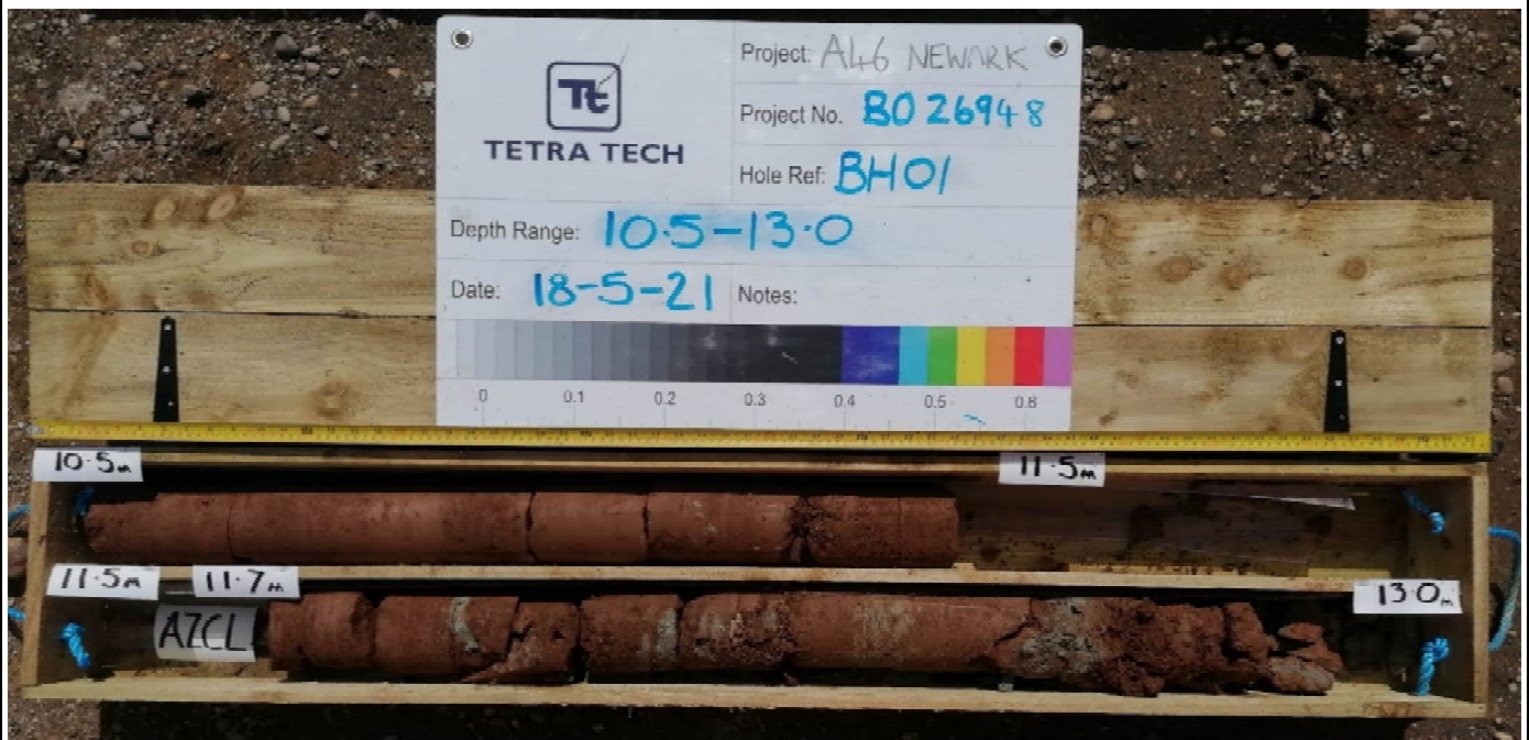
Plate 3 BH01 - 10.50 to 13.00m bgl
